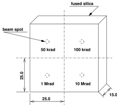
Figure 1: Schematic drawing of fused silica sample with irradiation spots.
